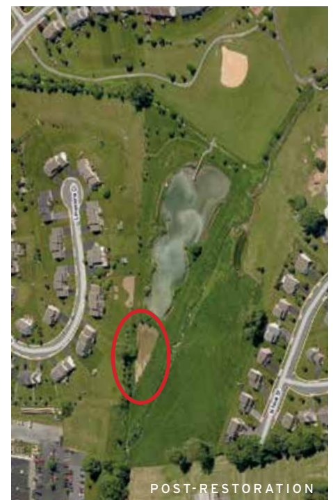
Water in the pretreatment settling basin (circled area) is brown with sediment. In the wetland above it, the water is noticeably cleaner.
